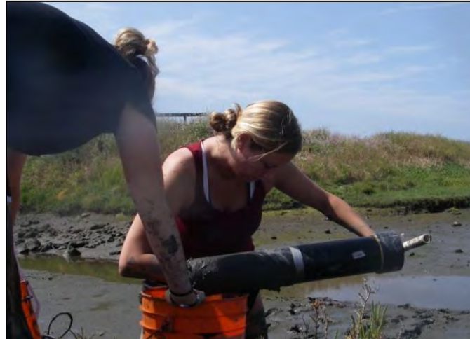
Figure 3. Example of large core sediment extraction.
