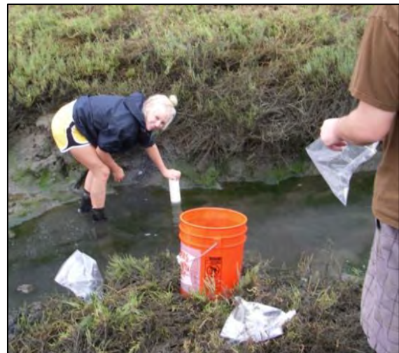
Figure 5. Small core pushed into the sediment.
