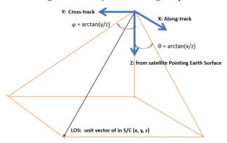
**Figure 6.** The OMPS LOS vector is expressed in the spacecraft coordinate, where the along-track (x-z plane) and cross-track planes (y-z plane) are formed. Two angles of  $\theta$  and  $\varphi$  simultaneously correspond to the unit vector of **LOS**.
