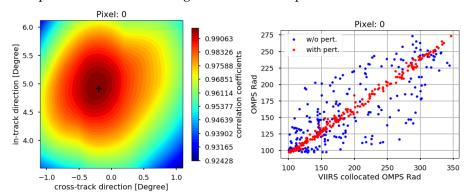
**Figure 9.** Contour plots (**left**) of the correlation coefficients between VIIRS-collocated and real OMPS-NM radiances varying with the perturbation angles in the along-track and cross-track directions for macropixel FOV 0, where the plus marker shows the maximum correlation coefficient. A scatter plot (**right**) between VIIRS-collocated and real OMPS-NM radiances with and without LOS vector perturbation.
