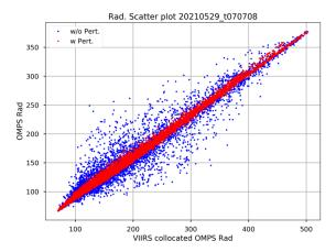
**Figure 5.** Scatter plot between real and VIIRS-collocated OMPS-NM radiances. The blue dots indicate the VIIRS-collocated OMPS-NM radiances using the original OMPS geolocation fields, while the red dots are perfectly aligned with the VIIRS. The radiance unit is  $W/(cm^3 Sr)$ .
