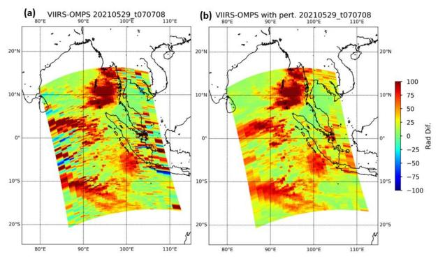
**Figure 4.** Radiance difference image between real and VIIRS-collocated OMPS-NM radiances: (a) based on the original OMPS geolocation fields and (b) the ones with perturbation that perfectly are aligned with VIIRS. The radiance unit is  $W/(cm^3 Sr)$ .
