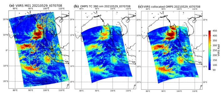
**Figure 1.** (a) VIIRS image at the M01 band (412 nm) on 29 May 2021; (b) the correspondent OMPS-NM image at 380 nm; (c) VIIRS-collocated image based on the OMPS-NM geometry characteristics. The radiance unit is  $W/(cm^3 Sr)$  in the images.
