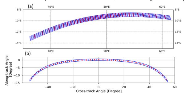
**Figure 3.** Example of OMPS-NM macropixel FOV shapes projected (**a**) on the Earth Surface, shown as longitude and latitude and (**b**) on the S/C coordinate expressed in the along-track and in-track angles (indicated by the bluelines). The red dots point to the FOV center. The FOVs on the Earth's location in five scanlines return to identical locations on the S/C coordinate after the inverse geolocation computation.
