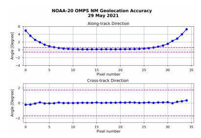
**Figure 11.** Geolocation assessment results, including the offset angles in the along-track and cross-track directions, where the dashed lines indicate the  $\pm 1/2$  macropixel FOV size in terms of degrees.
