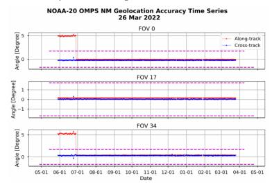
**Figure 13.** Time series of the assessment results for NOAA-20 OMPS-NM at macropixel FOV 0, 17 and 25, where different y-axis scales are used for three plots. The dashed lines indicate the  $\pm 1/2$  FOV size in terms of degree. The time series extended from 27 May 2021 to 26 March 2022 (309 days) and the data in each day contains 150–200 OMPS-NM lines with randomly selected non-uniform scenes.
