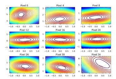
**Figure 10.** Contour plots of the correlation coefficients between VIIRS-collocated and real OMPS-NM radiances varying with the perturbation angles in the along-track and cross-track directions at the nine (9) macropixel FOV positions, where the angle values with the maximum correlation are used to estimate the geolocation error of OMPS-NM.
