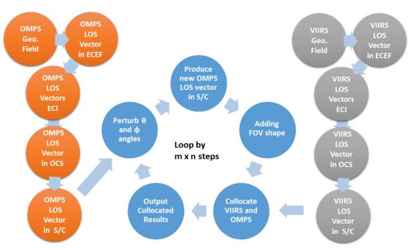
**Figure 12.** Flowchart describing the method of quantifying OMPS-NM geolocation accuracy using VIIRS M1 band geolocation data.
