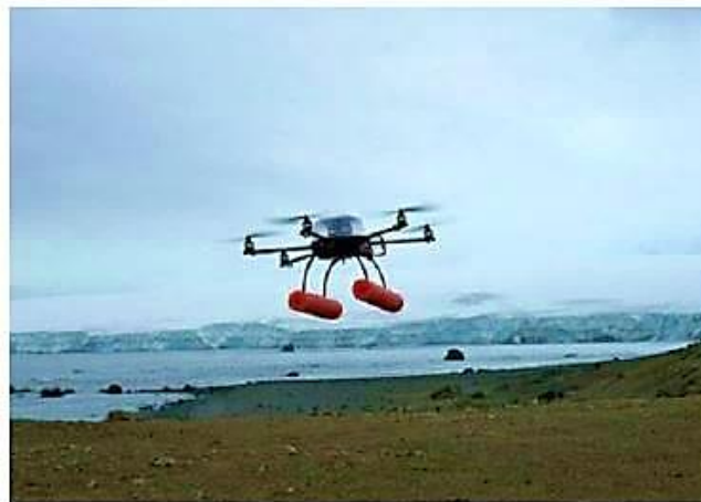
Figure 9. One type of unmanned aerial system that has been used in the field by NOAA/NMFS personnel for marine mammal research: the APH-22 Hexa-copter.
