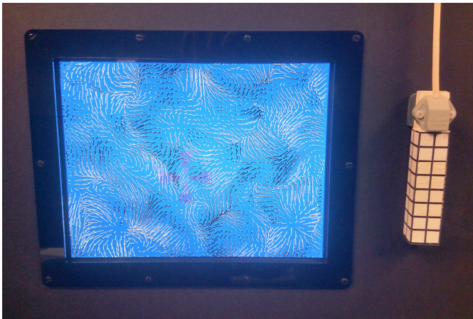
Fig. 2. The experimental apparatus, consisting of a 25cm diagonal high-resolution "Retina" display and an electromagnetically tracked hand-held probe for inputting perceived orientation.
