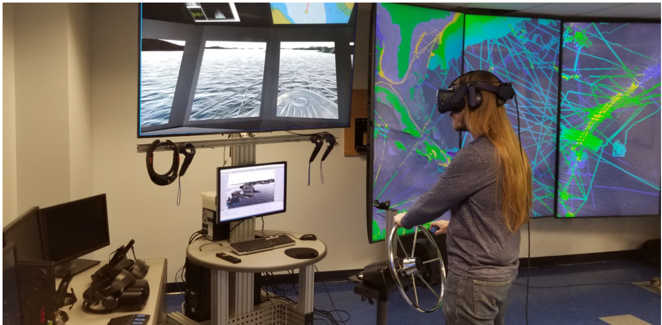
Figure 1: The experimental setup. Participants wear a head mounted display while interacting with physical boat controls (wheel and throttle). A television provides a mirror view that allows experimenters to monitor subjects’ performance.
