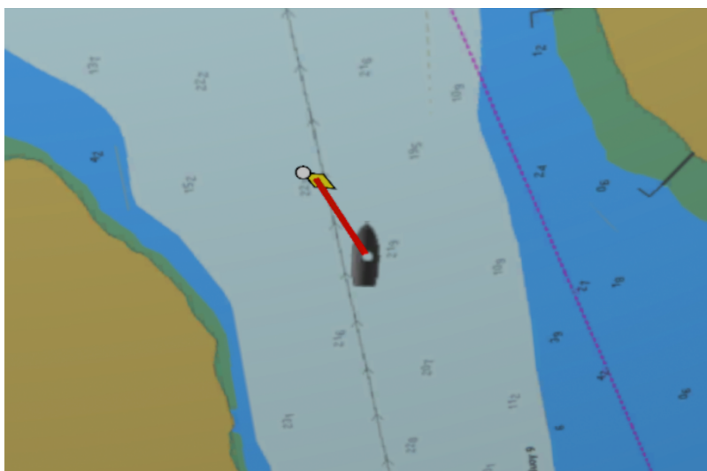
Figure 4: Detailed view of the track-up ECDIS display in the simulation, showing target buoy (yellow icon) and connecting line (red) between boat and target. The chart automatically pans and rotates to keep the boat in the center and facing upward.
