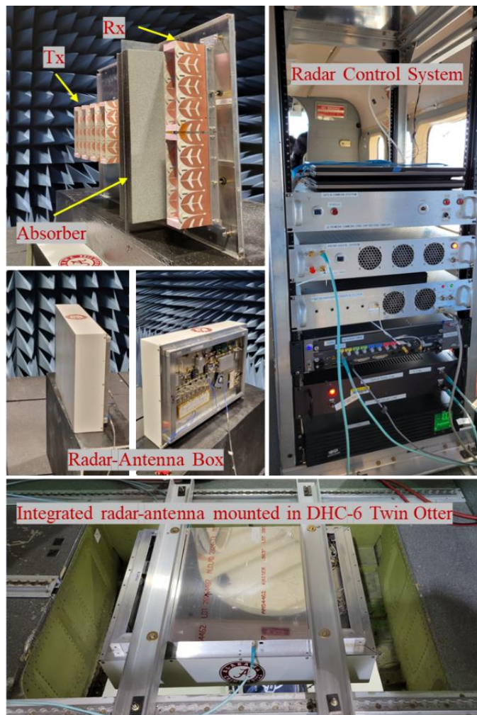
Fig. 11. Antennas-radar integrated unit during anechoic chamber test and radar control system rack mounted on DHC-6 Twin Otter aircraft.
