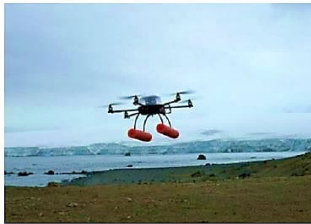
Figure 25. One type of unmanned aerial system that has been used in the field for marine mammal research: the APH-22 Hexa-copter.
