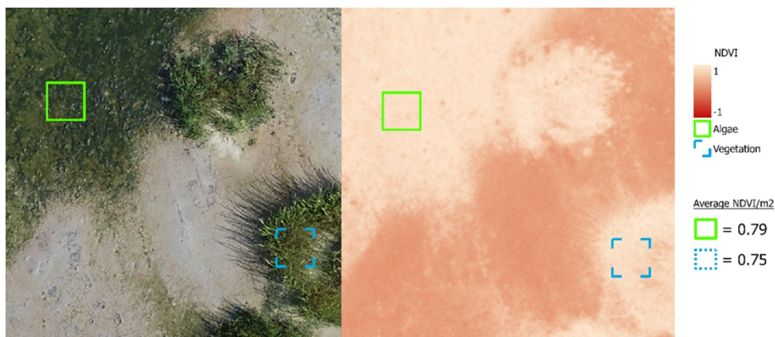
Figure 17. Overlap in NDVI values between benthic periphyton and S. alterniflora complicates imagery-based quantification of vegetative biomass. Left panel = RGB imagery, Right panel = NDVI raster.
