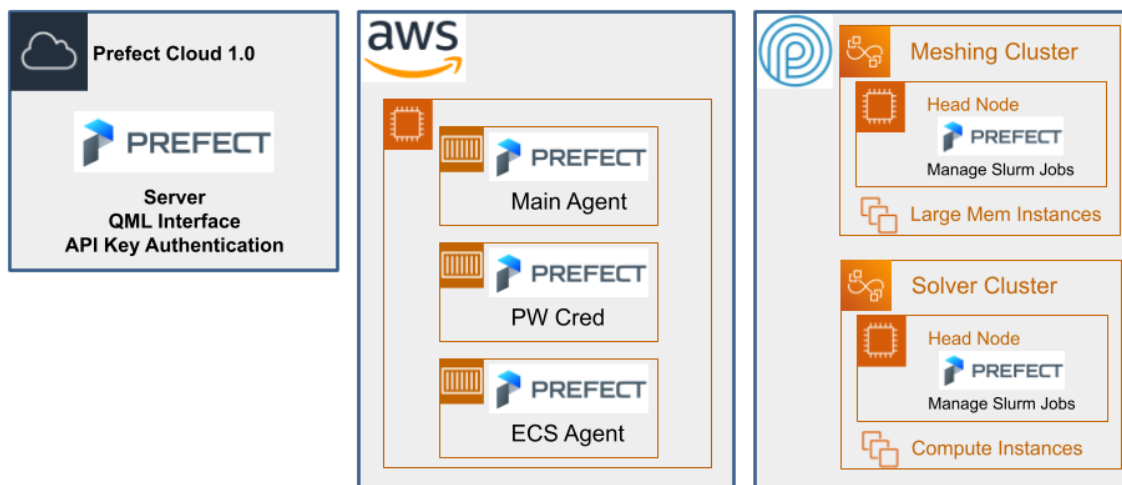
Figure 8 Arrangement of Prefect agents for the workflow system
