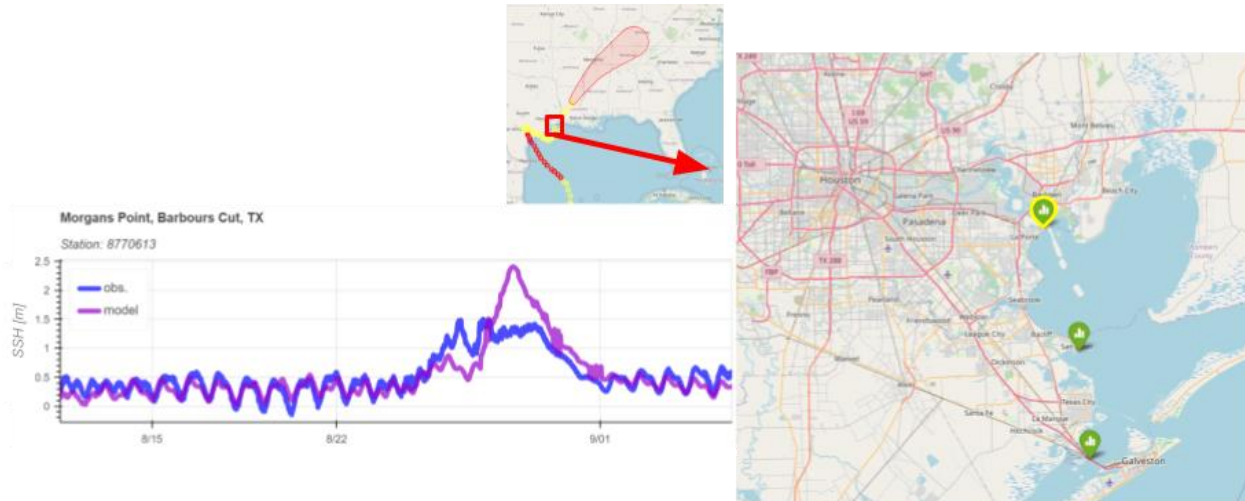
Figure 15 Comparison of measurement and simulation time series at Morgan's Point station in Texas for Hurricane Harvey (2017). The bias is removed to only emphasize on the signal of the storm
