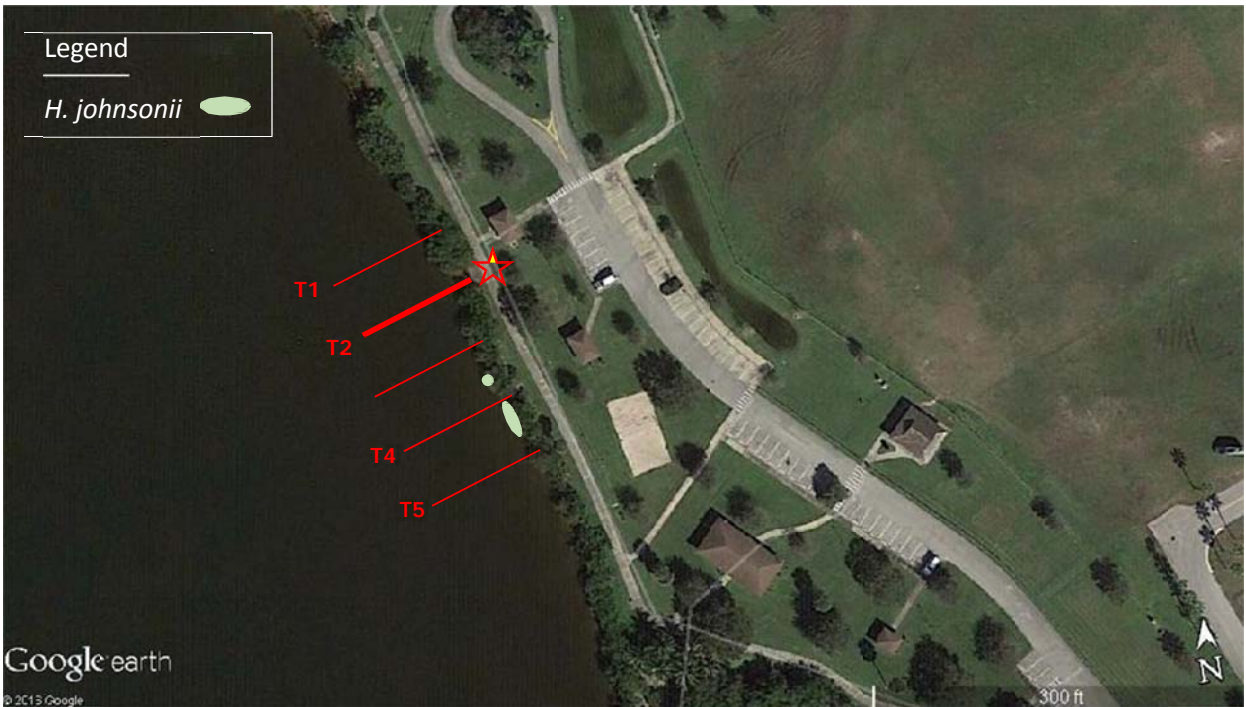
Figure 3.1. April 13, 2016, SAV survey transects with results. Transects spaced approximately 50 feet apart (not to scale). T2 transect is proposed fishing pier location; there was a secondary possible location at T4, which was eliminated due to presence of Johnson’s seagrass (Corps consultation package).
