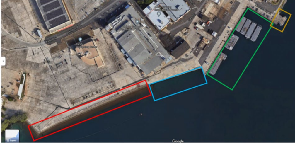
Figure 15. The conceptual plan for construction support facilities at FI: (red) off-limits; (blue) Access Area for loading/unloading; (green) temporary pile clusters for loading/unloading and barge storage; and (brown) loading/unloading (source: NAVFAC 2022a).
