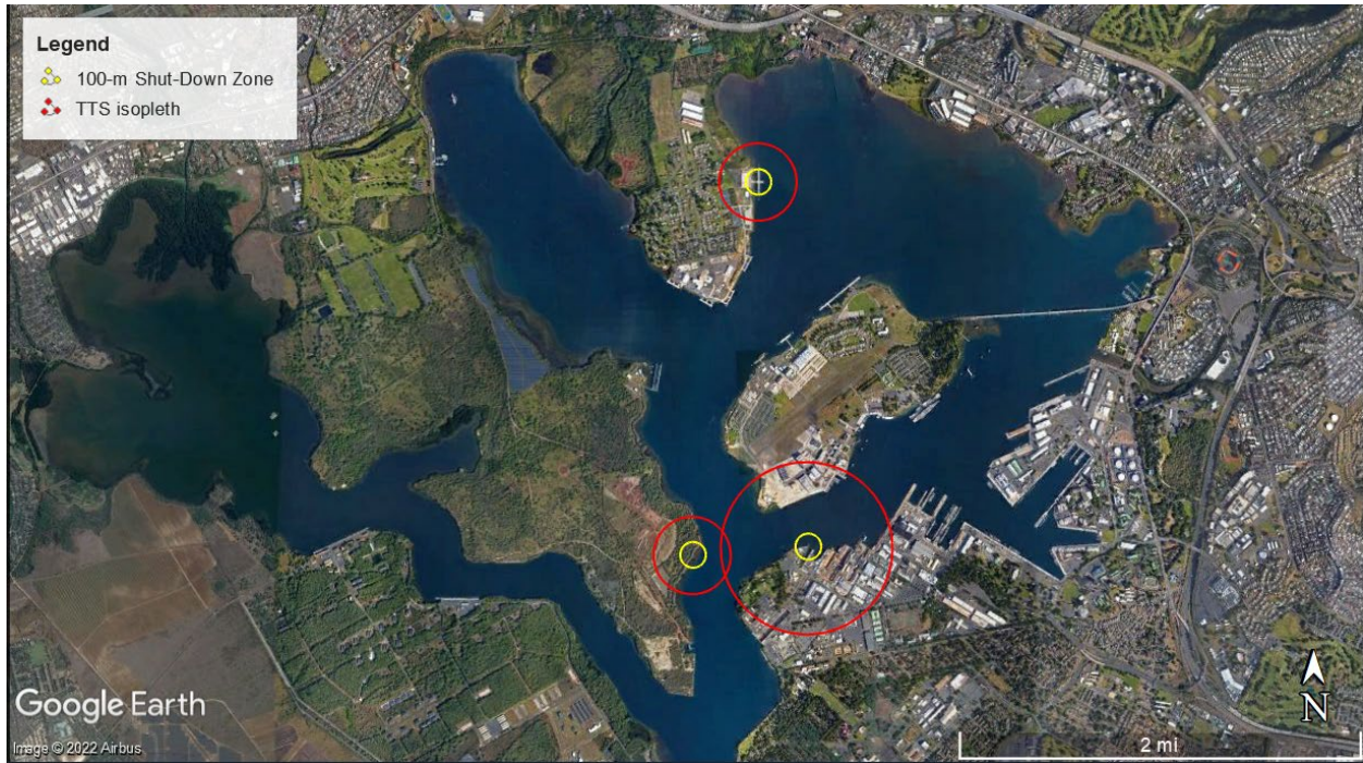
Figure 28. Effect distances to TTS thresholds (189 dB SELcum) from impact driving of 36-inch steel pipe piles, 42x18-inch H-piles, and 18x18-inch H-piles, and 100-m shut-down zones at PHNSY & IMF, WP and PCP.
