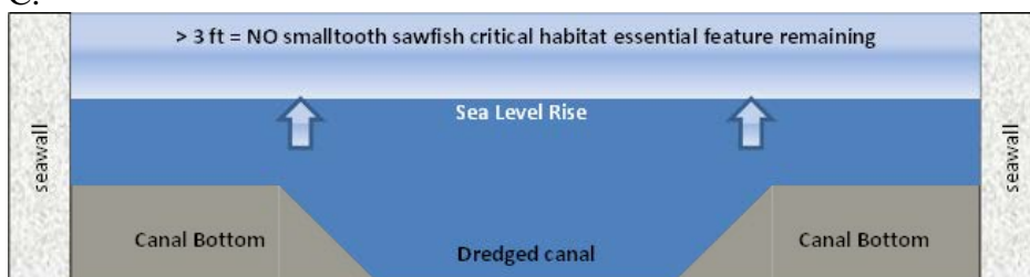
Figure 4. Diagram A depicts a cross section of a historically dredged channel/canal within the boundaries of the critical habitat units that has not been maintained. Diagram B depicts the typical cross section of a
