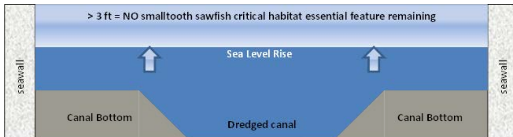
Figure 6. Diagram A depicts a cross section of a historically dredged channel/canal within the boundaries of the critical habitat units that has not been maintained. Diagram B depicts the typical cross section of a maintenance dredged channel/canal. Diagram C depicts a cross section of a maintained dredged channel/canal after sea level rise of > 1 ft.
