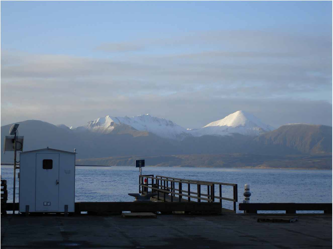
Acoustic tide gauge station located at Sand Point, Alaska. Tide gauges are used to measure the arrival time and maximum amplitude of a tsunami at the coast. Tide gauge data often provide the first confirmation that a tsunami was observed at the coast and are used for developing and validating tsunami forecast and inundation models. The U.S. National Ocean Service operates over 180 tide stations that have been upgraded to enable the collection and dissemination of 1-minute data. Photo credit: NOAA/NOS.
