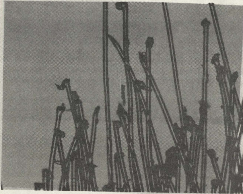
FIBER 4.1-10 Test sample (530 feet above bottom chain) sawed on metal under low tension. (64X)
