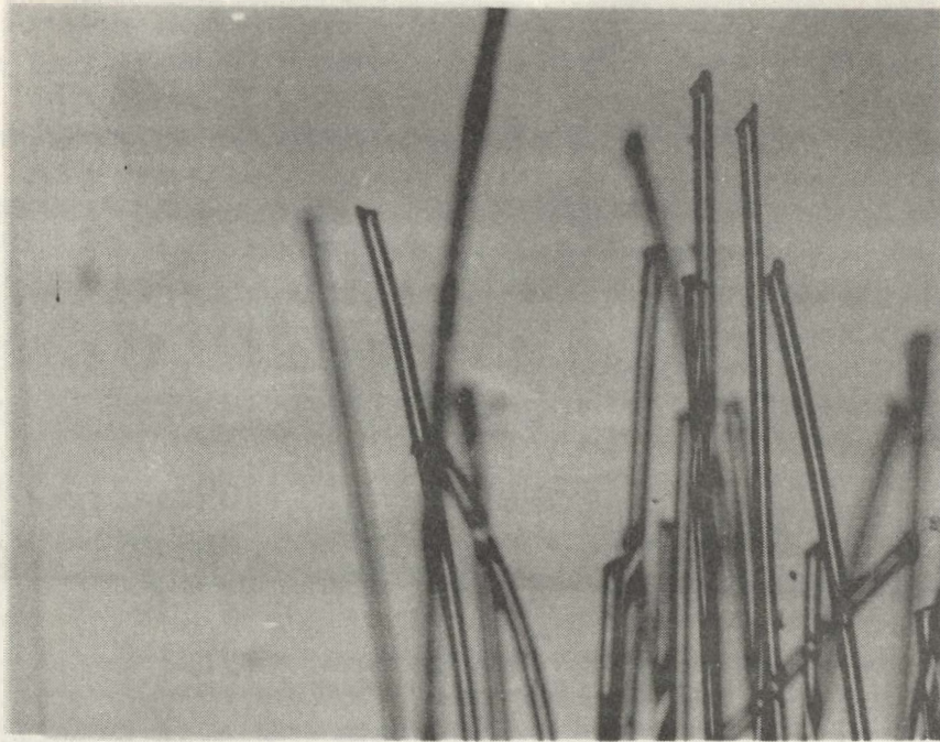
FIGURE 4.1-5 Photomicrograph (64X) of fibers from fishbite at 650 feet below SCI Buoy E (taken from outer cover strands)
