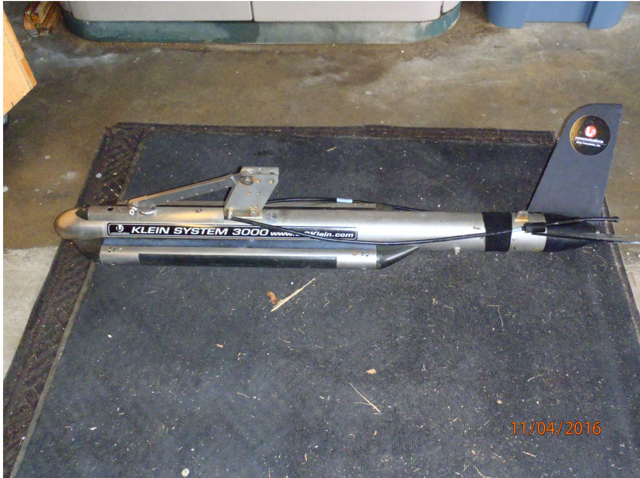
Figure 2.1. Klein System 3000 (model #3200)™ Side Scan Sonar transducer that is towed behind the 45 foot R/V Marguerite (from USFWS consultation initiation package).
