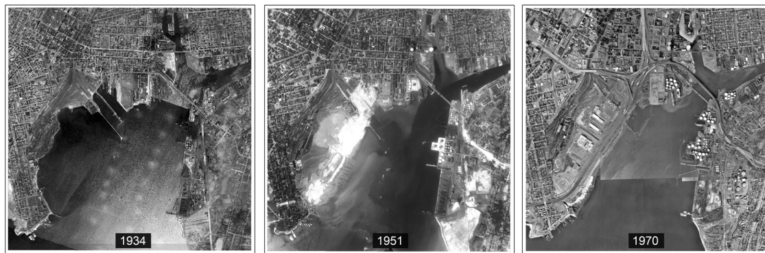
Fig. 2 New Haven harbor area changes from 1840s to 2010s. Left: New Haven harbor in 1934. Middle: Long Wharf under construction in 1951. Right: Long Wharf industrial area and the interstate transportation system formed under dramatic coastal landfills
