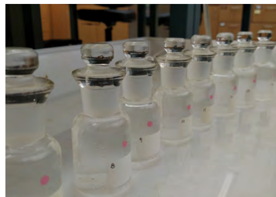
Optode bottles used in incubations to estimate rates of pelagic planktonic respiration. Photo: Jude Apple
