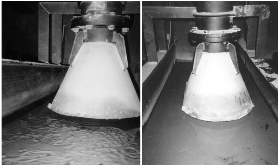
Figure 3-1: The bottom edge of the intake/pump-out port (bellmouth) in ballast tanks must be positioned far enough off the bottom deck plate to achieve the high flow rates required to fill and empty the tank (Photo courtesy of the Great Lakes NOBOB Assessment Project).
