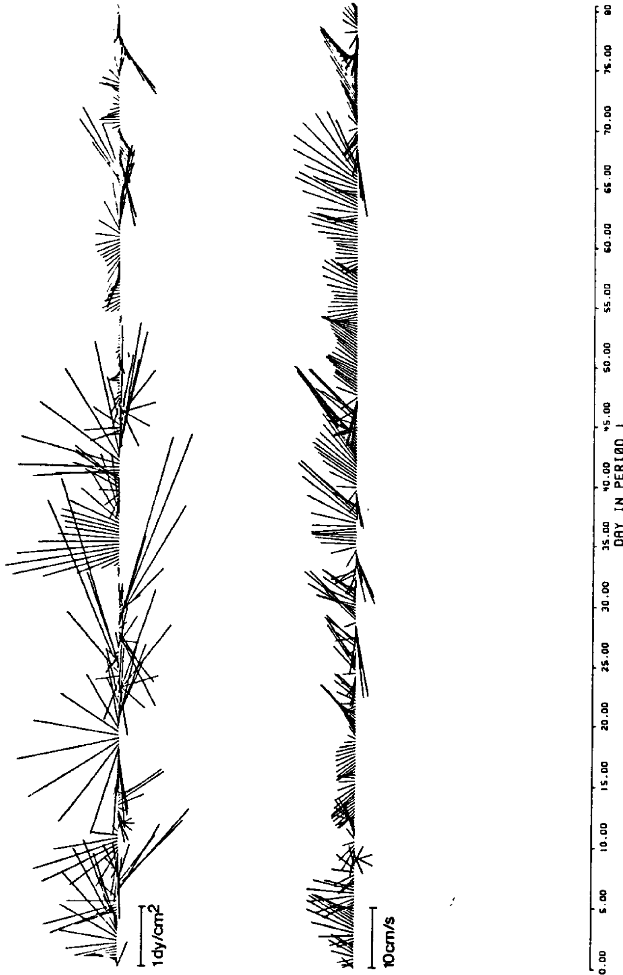
Figure 4a. Period 1, 21 February - 13 May 1977. Stick vector plot of 40 hr low-passed wind stress (dyne/cm 2 ) and current (cm/s) at SNLT. North is toward top of figure.
