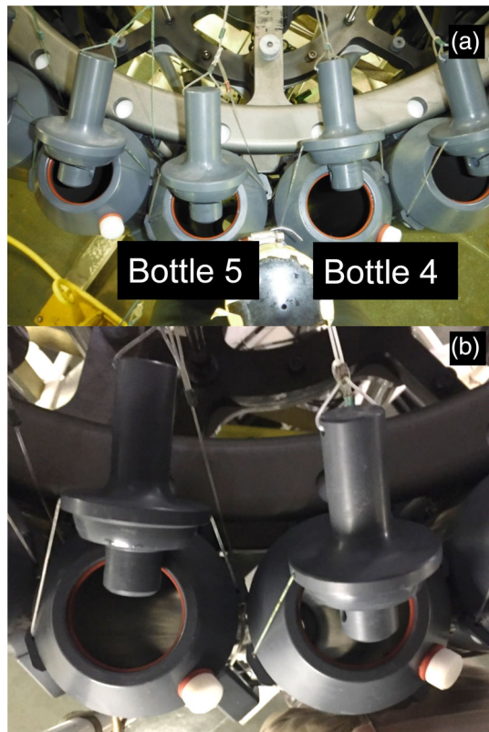
Fig. 14. Photos showing (a) cocked bottles on HLY201301 showing variations in bottle openings, and (b) the top view of the two cocked bottles for the end plug cocking experiments during cruise HLY1702.
