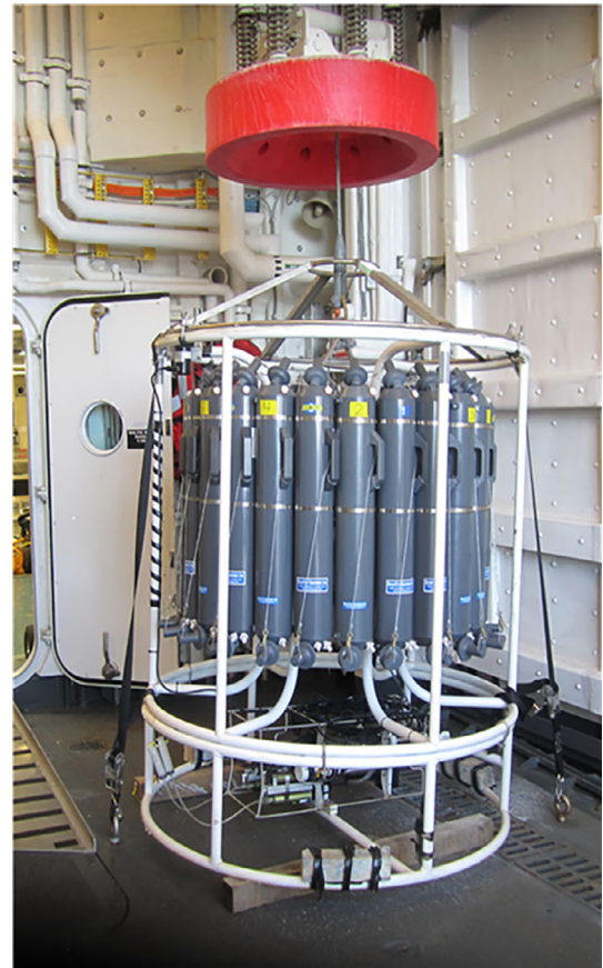
Fig. 6. Carousel system employed on the RV Sikuliaq .
