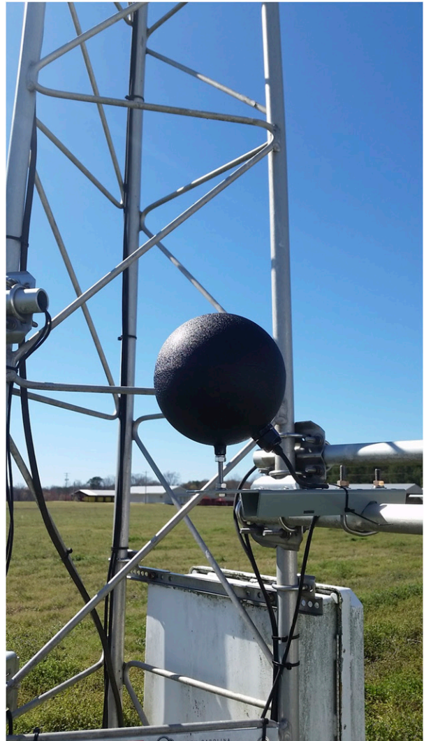
FIG. 1. Black-globe thermometer installed at the North Carolina ECONet Site in Rocky Mount, North Carolina. The image was provided by the NCSCO.
