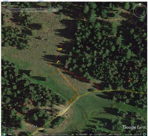
Figure 19. Temp road 005444 (red line) aquatic design features. Thick yellow lines = waterbars, thin brown lines = wood obstructions.
