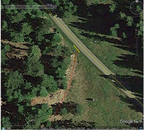
Figure 18. Temp road 0025288 (red line) aquatic design features. Thin yellow line= waterbar, thin black line=silt fence
