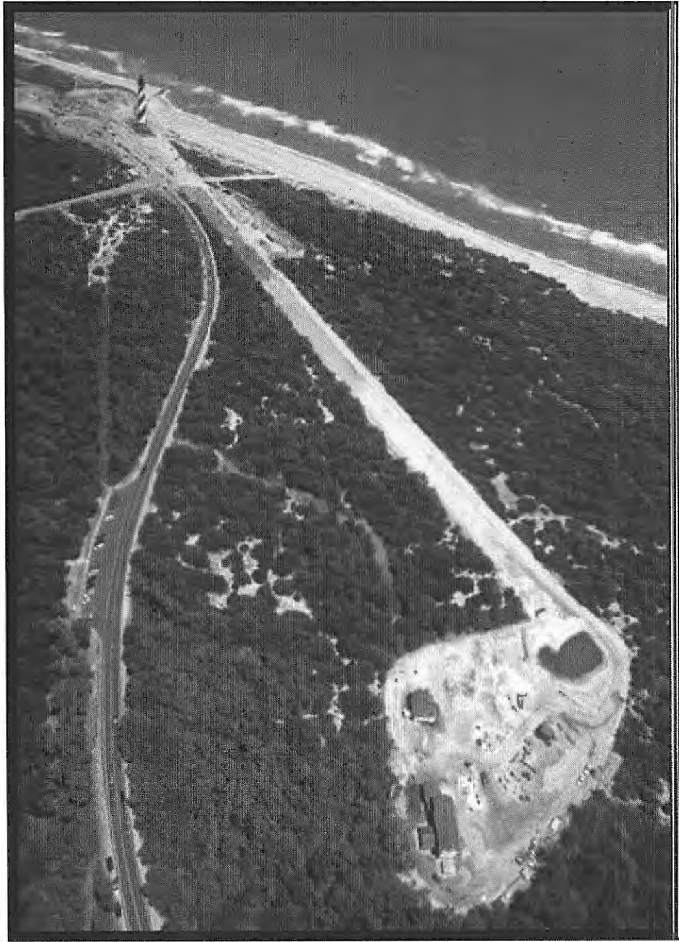
Figure 1-33. Cape Hatteras Lighthouse is being prepared for its move from the old threatened site adjacent to the rapidly eroding shoreline to a new inland site. Photograph is by the N.C. Department of Transportation.
