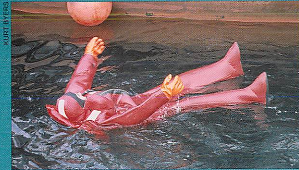
The life-saving orange-red "Gumby" suit is made of closed-cell foam rubber.
