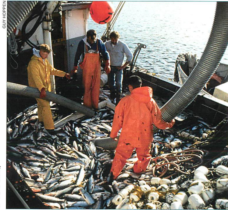
Pink salmon on the deck of a purse seine boat are sucked into a ten-inch hose by a fish pump onboard a tender tied up to the seine boat.
