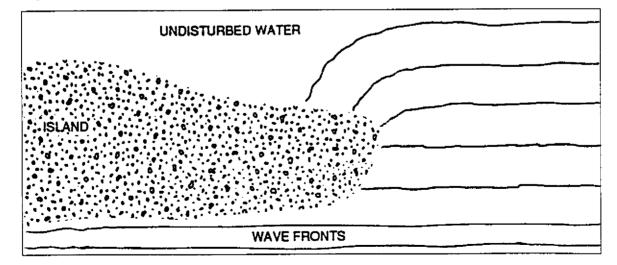
Figure 5. Wave Diffraction.
