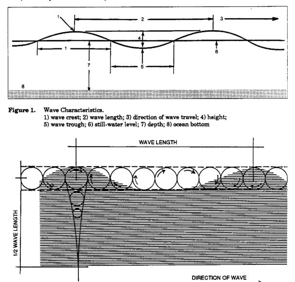
Figure 2. Cross-Section of Wave (traveling from left to right). Circles represent water particles in the wave.
