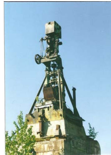
Figure 5. Photograph of last standing steam stamp at the remains of the Ahmeek stamp mill in Tamarack City. (1990)
