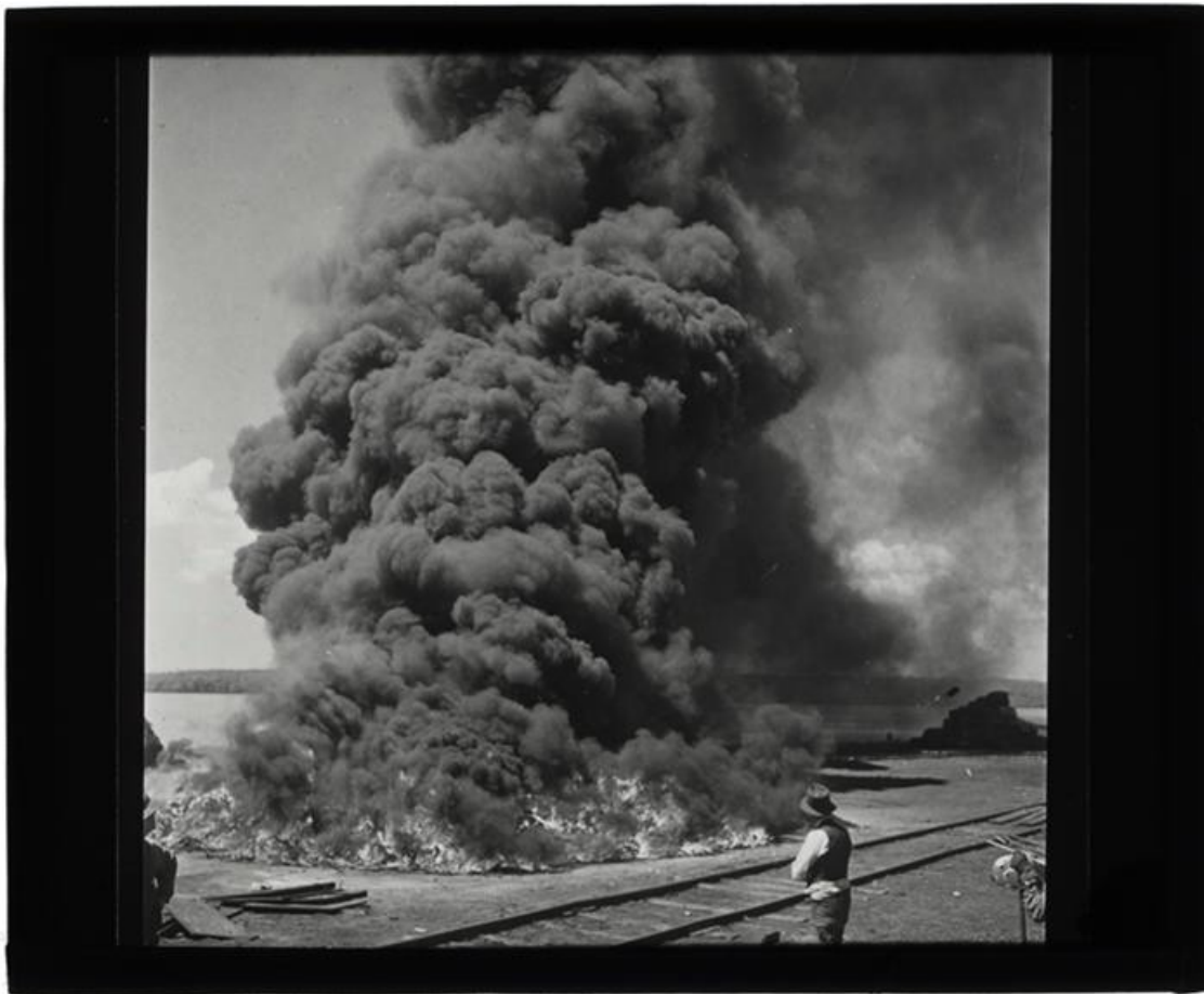
Figure 2-4. Burning of Copper Scrap in C&H Hubbell Smelter Yard (circa 1950s). Courtesy: Keweenaw National Historic Park Archives.
