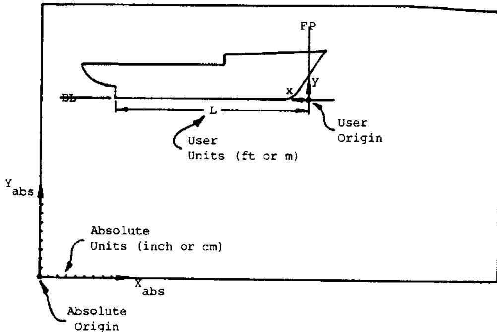
Figure 2. Absolute and user-defined coordinate systems. In this case, the user origin for the profile is defined as the intersection of the baseline and fore perpendicular. Note also that the positive x direction in the user-coordinate system is directed to the left, since the bow is drawn to the right. In many systems, this reversal of direction is achieved by entering a negative scale factor.
