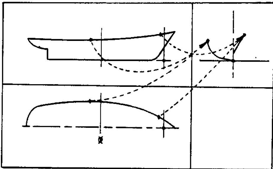
Figure 6. Direct three-dimensional definition of an object on the digitizer. A point entered at a specified station in both profile and half-breadth views is located in three dimensions, and shown in the body plan. For the usual graphic format of the body plan, special additional programming is required to cause the display of the forebody on one side of the centerline, the afterbody on the other.
