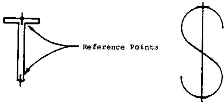
Figure 7. Typical macros. The valve assembly macro is shown as a simplified three-view drawing, permitting the macro to be entered in any orthogonal view. Advanced systems may also permit general rotation of the macro before insertion into the main drawing, although automatic hidden line removal is generally not available. The structural cross-section and weld symbol are simple two-dimensional macros.
