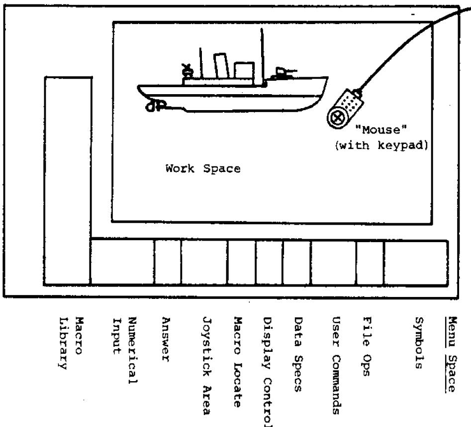
Figure 5. Work space and menu space, shown on a digitizer board. The menu regions shown are similar to those of the GCADS graphic design system, currently implemented on PDP-11 minicomputers. (Adapted from C.R. Besant, Computer-Aided Design and Manufacture, 2nd Ed., Ellis Horwood, Chichester, England, 1983.)
