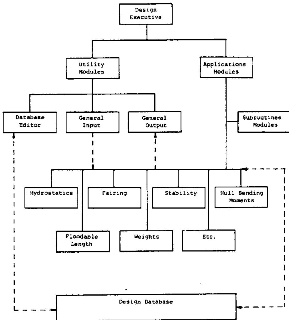
Figure 1. Structure of a typical design system. In this diagram, control functions are shown by solid lines, while dotted lines indicate the flow of design data. Each individual module shown by a single block is generally loaded into RAM separately. Thus, the over-all size and complexity of the system is limited by disk-storage considerations rather than by RAM capacity. However, the complexity of each individual module is constrained by RAM.
