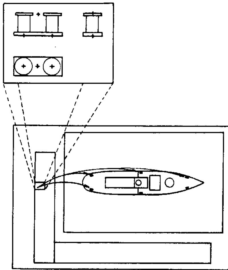
Figure 8. Installation of a macro (a double mooring bit) on a deck layout. Each location of the macro is achieved by fixing one of the macro reference-point locations on the drawing, and specifying a line segment to give the angular orientation of a second reference point.
