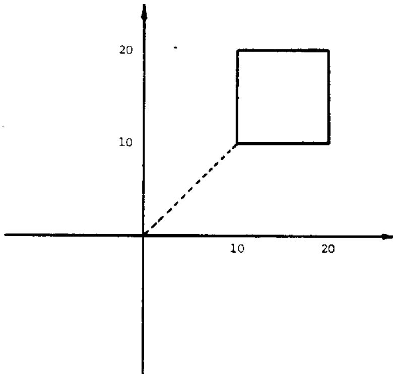
Figure 4. Trailing-origin cursor movement. The cursor begins at the origin, (0,0). The command sequence is identical to that of Fig. 3. In this case, however, each cursor movement corresponds to a vector beginning at the current position of the cursor.
