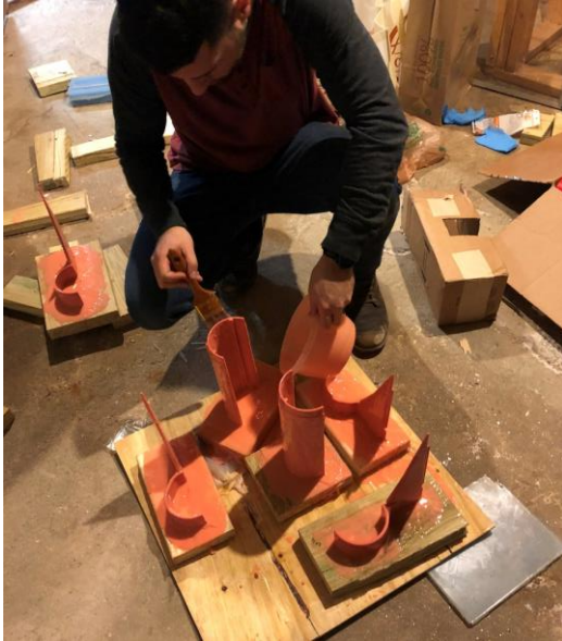
Figure 20: Application of the brush-on silicon mold
