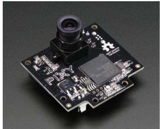
Figure 23: HD camera with a built-in processor
