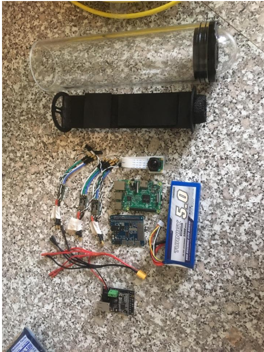
Figure 14: Watertight enclosure and electronics
