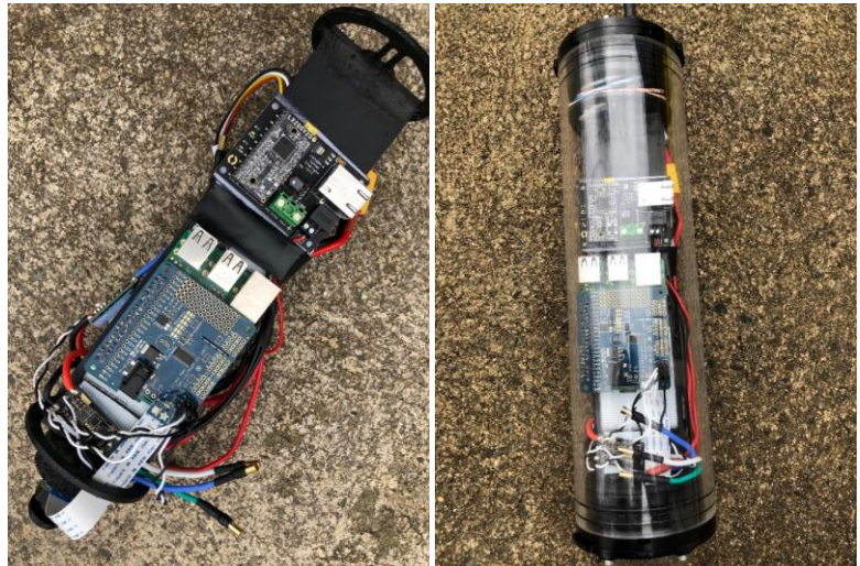
Figure 16: Assembled electronics tray (left) Assembled electronics tray inside waterproof enclosure (right)
