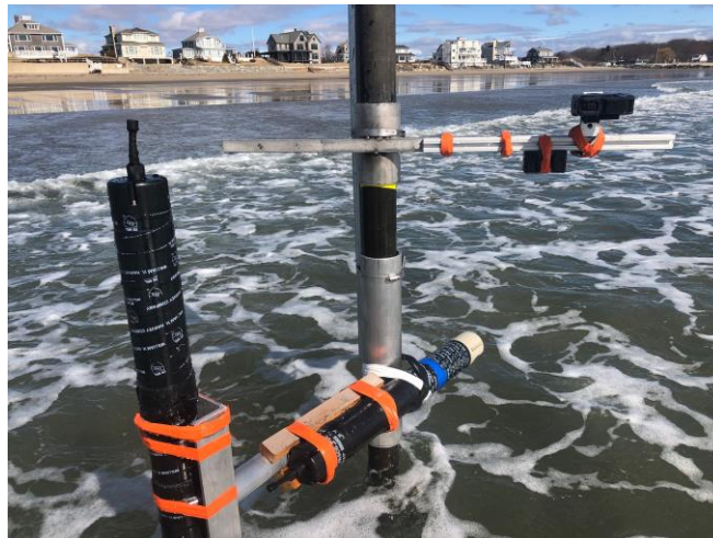
Figure 22: The field deployment set up. The instrument mount with the ADV and Aquadopp attached sit on the lower part of the jetted pipe. The camera is mounted to the field deployment frame, above the instrument mount, positioned straight down.
