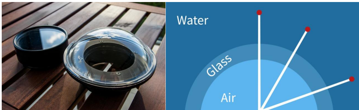
Figure 24: Left – The difference between a dome port and a flat port [12]. Right – Dome ports are unaffected by refraction and can remove distortion associated with capturing images underwater [12].
