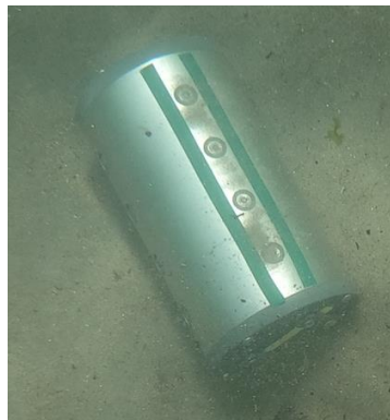
Figure 20: The Pressure Mapped Munition (PMM) underwater during deployment on April 14, 2019 at Wallis Sands.
