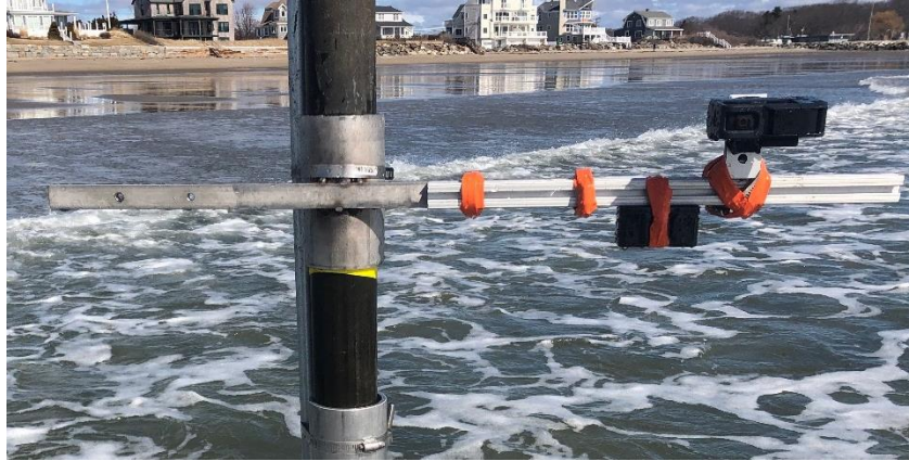
Figure 3: The field deployment frame in use at Wallis Sands Beach, New Hampshire. The cuff is secured on a jetted pipe, and the camera is extended on the mount away from the jetted pipe positioned with the lens facing straight downwards.
