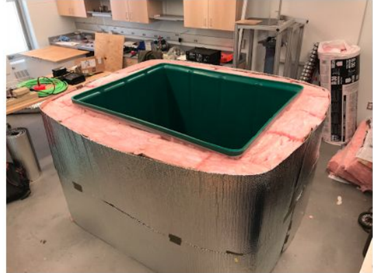
Figure 18: The tank and insulation attached to the sides of the tank for design version 2.
