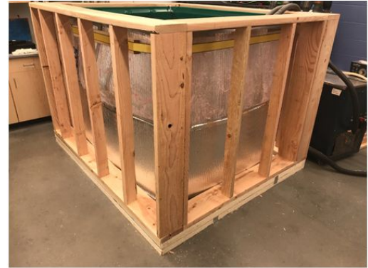
Figure 23: Final insulated base and frame
