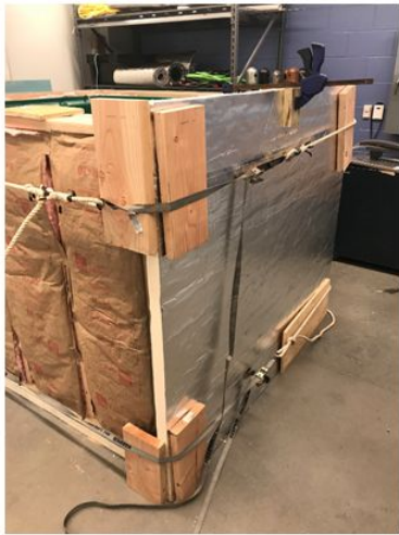
Figure 24: Assembly of outer insulation
