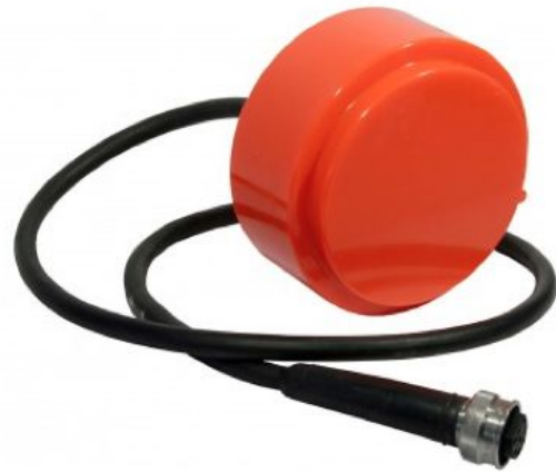
Figure 9: The Simrad ES200-7CD transducer used throughout this experiment ( https://www.simrad.com/www/01/nokbg0240.nsf/AllWeb/3ADE61D37DE79B37C12575430040FE22?OpenDocument )
