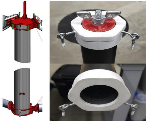
Figure 2: Comparison between the top and bottom caps and joints of the full-scale and the actual model.
