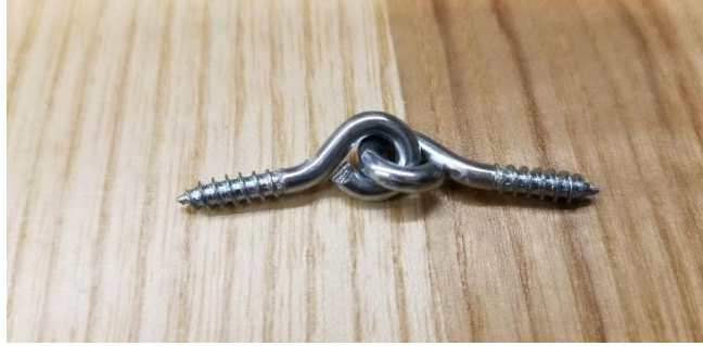
Figure 5: Scale model screw eyes used to simulate the bottom joints of the full-scale cage.
