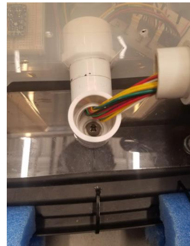
Figure 20: Sensor tower tube with ultrasonic sensor wires going through it
