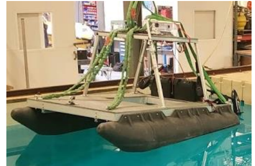
Figure 21: ASV in engineering tank
