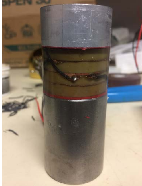
Figure 20. Transducer casted in urethane
