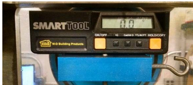
Figure 10: Electronic level setup with calibration block
