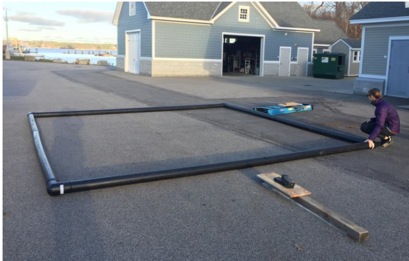
Figure 9: The welded HDPE frame.
