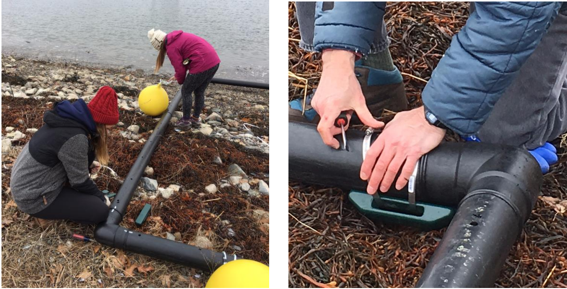
Figure 17: (left) Attaching buoys and weights to the frame on the beach. (right) A close-up of the dive weights being fastened to the corner of the frame using hose clamps.
