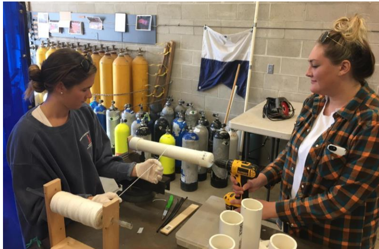
Figure 12: Preparing the spools using a drill to spin the PVC pipe, while the twine was guided onto it.
