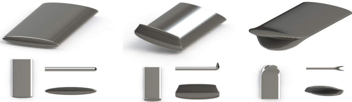
Figure 1: Images of End Cap Foil (left), General Foil (middle), Split Tip (right).
