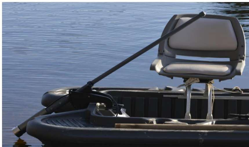
Figure 16 Sonar system with mount in storage position.
