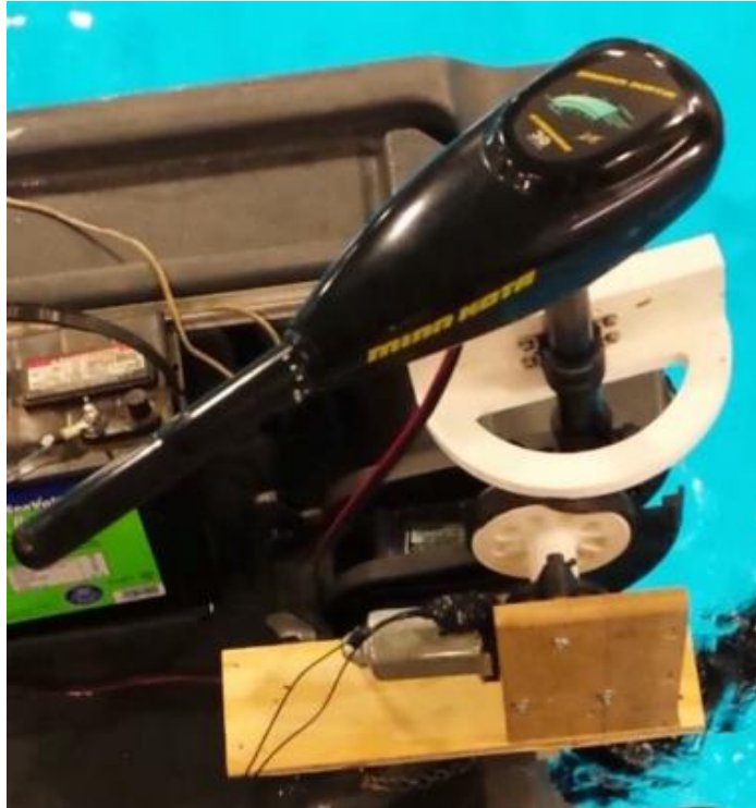
Figure 6: Assembled steering system being tested on ASV in UNH Chase Ocean Engineering Laboratory pool
