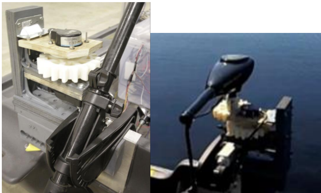
Figure 9: Revised steering system design. Left: Motor disengaged and stored. Right: Motor engaged.
