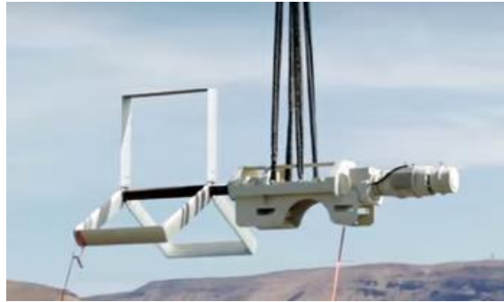
Figure 2- Instream Cross-Flow Turbine in Roza Canal, Washington
