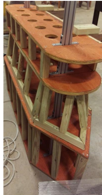
Figure 6- Froude scaled Model of Bridge Pier in Progress
