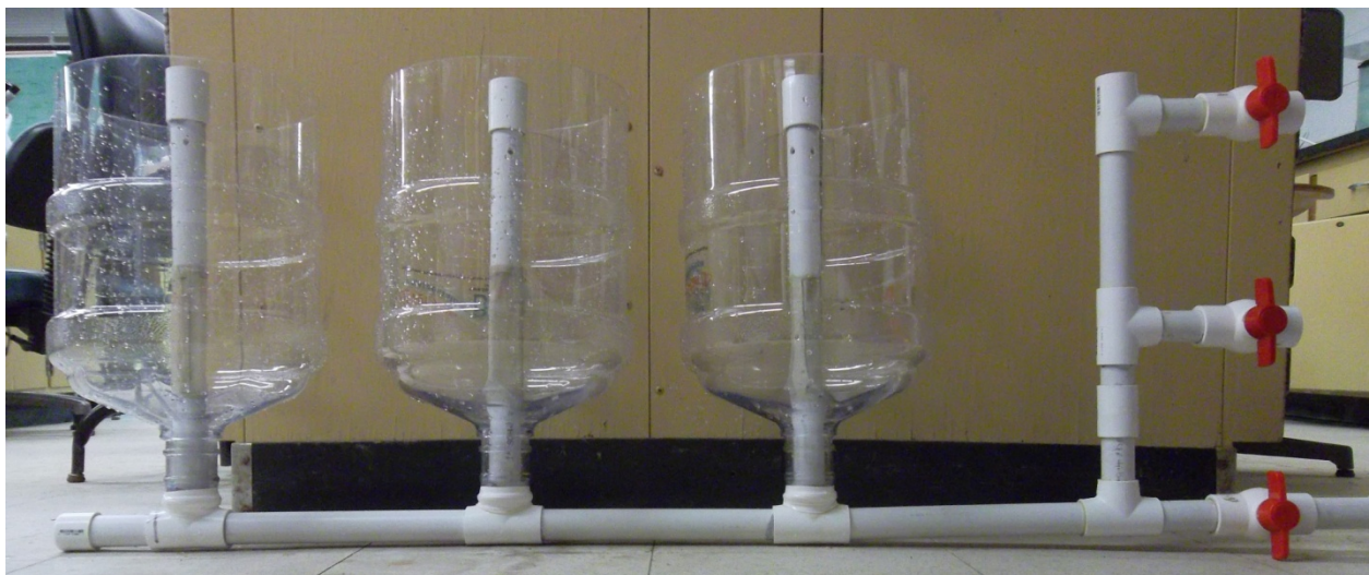
Figure 7.3 - A three tank set connected to outlet valves
