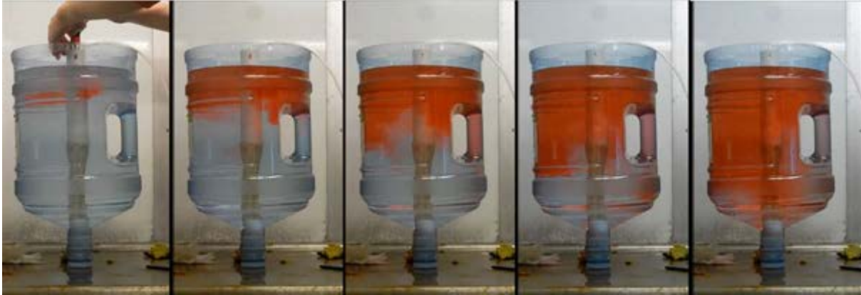
Figure 8.3 - Dye flowing through the central pipe's outlet holes
