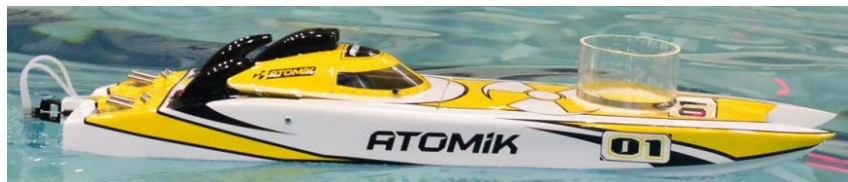
Figure 1-Boat used as ASV platform.
