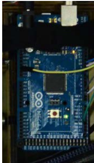
Figure 2-Arduino used for motor and rudder control.
