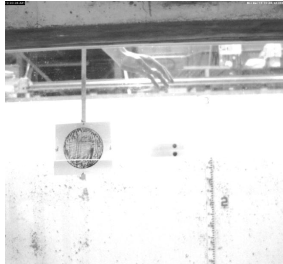
Figure 4: OPIE image of the 1/10 th scaled model buoy with the black dots used for tracking.
