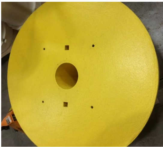
Figure 7: Picture of the buoy float showing the inner diameter hole, the 4 slotted rod holes, and the 2 frame through holes.
