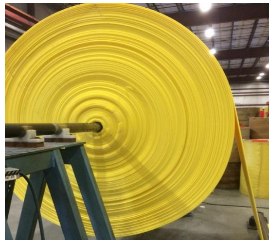
Figure 8: Photo from the fabrication process of the buoy float representing that foam sheets wound cylindrically to form the buoy shape.
