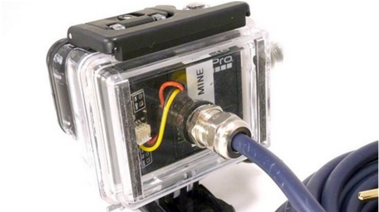
Figure 4: Video cable connected to custom GoPro housing (12V power cable included in final design) [1]
