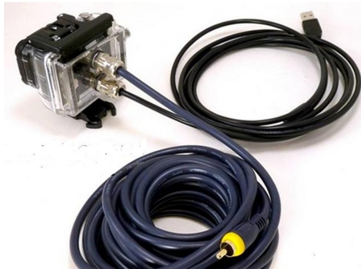
Figure 5: Video cable and 12V power cable coming out of custom GoPro housings [1]
