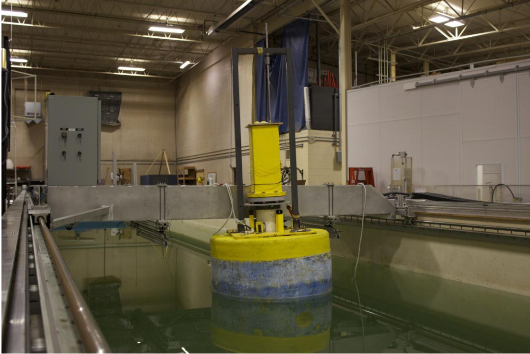
Figure 14: Photograph of the Wave Energy Conversion Buoy in the wave tank at the Jere A. Chase Ocean Engineering Laboratory.
