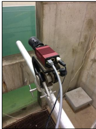
Figure 17: The OPIE camera pointed towards the window on the side of the wave tank.
