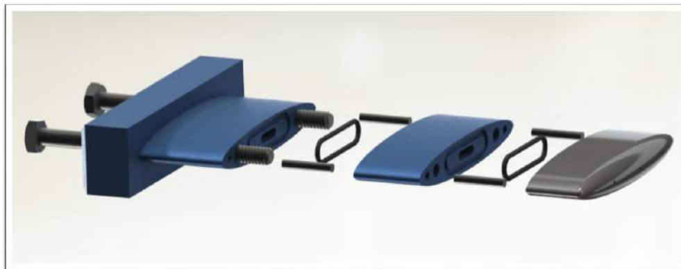
Figure 26: Exploded View of Experimental Apparatus. Left to Right: Base, Extension, EndCap (or other wingtip device).
