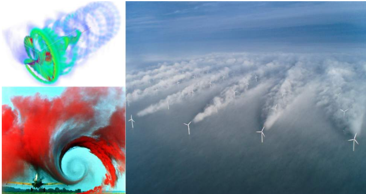
Figure 3: Top left: CFD analysis on wind turbine showing wake effects behind the turbine including wingtip vortices [8]. Bottom left: Wingtip vortex forming around airplane wing [7]. Right: Photographer Christian Steiness: The above photograph shows the turbulence field behind the Horns Rev 1 offshore wind turbines. Unique meteorological conditions on 12 February 2008 at 1300 hours resulted in the wind turbines creating condensation (i.e. clouds of the very humid air), thus making it physically possible to see the turbulence pattern behind the wind turbines” [8].
