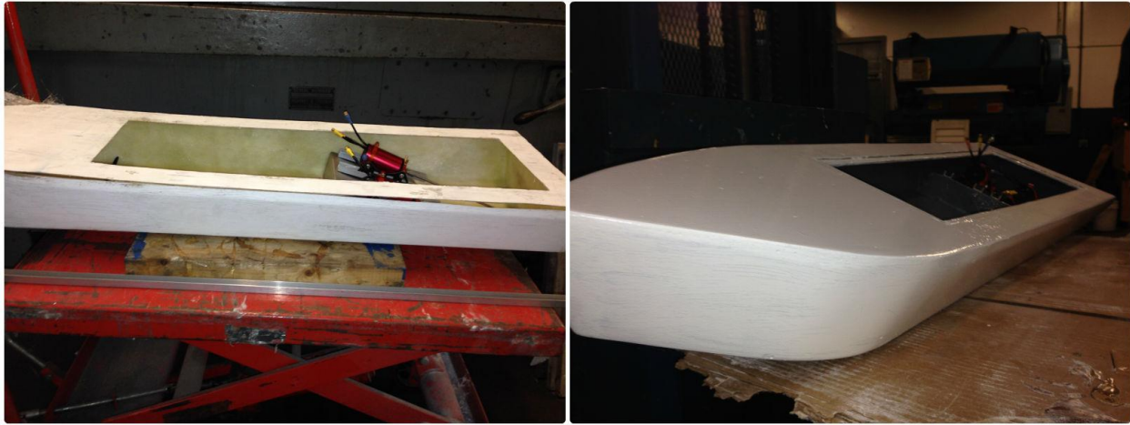
FIGURE 3: (LEFT) UNSEALED TOP AND BOTTOM HULL COMPONENTS. (RIGHT) SEALED TOP AND BOTTOM.
