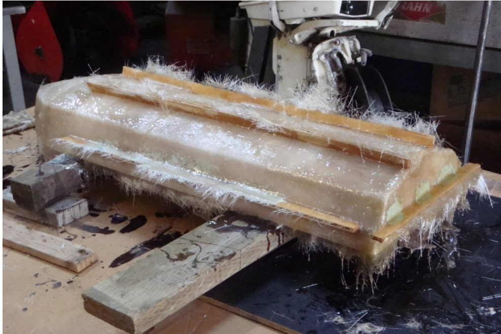
FIGURE 23: THE SECOND MOLD OF THE BOTTOM OF THE HULL. THE SURROUNDING CARDBOARD WAS IMPLEMENTED IN ORDER TO MAINTAIN THE STRUCTURAL INTEGRITY OF THE HULL DURING FIBER GLASSING AS IT TEND TO SHRINK AS IT DRIES.
