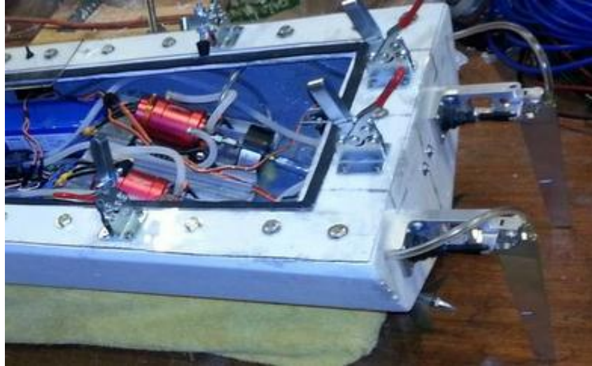
FIGURE 5: MOTOR AND RUDDER SETUP OF ASV.
