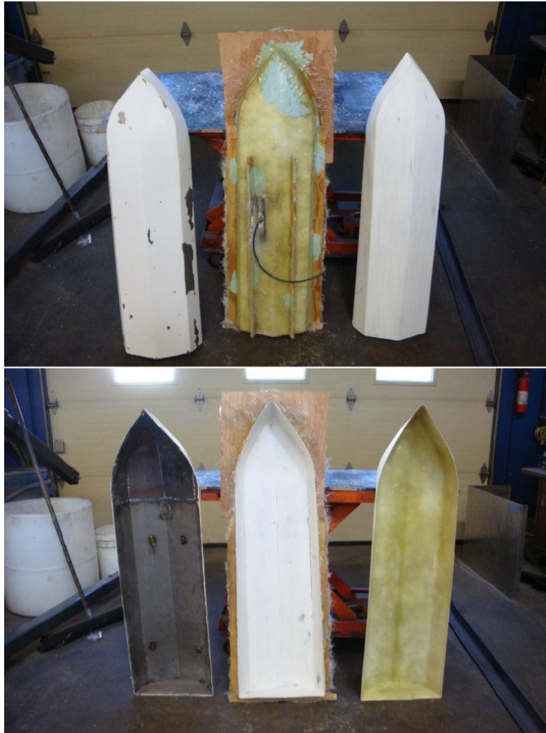
FIGURE 2: HULL CONSTRUCTION PROCESS. FROM LEFT TO RIGHT, STEEL MOLD, FIBERGLASS MOLD, TO FINAL FIBERGLASS HULL.
