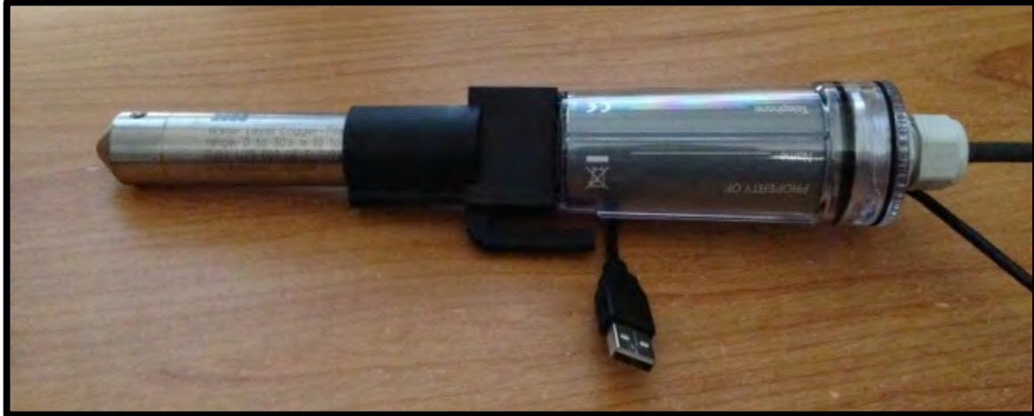
Figure 6: The pressure sensor attached to the computer connection device (HOBO U20 Titanium Water Level Data Logger - U20-001-02-Ti, 2012).
