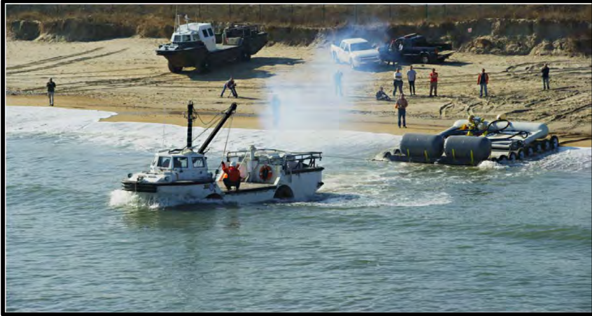
Figure 26: Deployment of a SurgeWEC device at the U.S. Army Corps of Engineers field research station in Duck, North Carolina on December 1, 2012. An Army surplus Ligher Amphibious Re-Supply Cargo (LARC) was used to tow the SurgeWEC into position. Moving the SurgeWEC from the beach to its final location took approximately 10 minutes (14).
