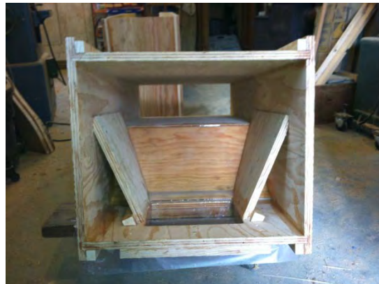
Figure 17: Top view of diffuser under construction
