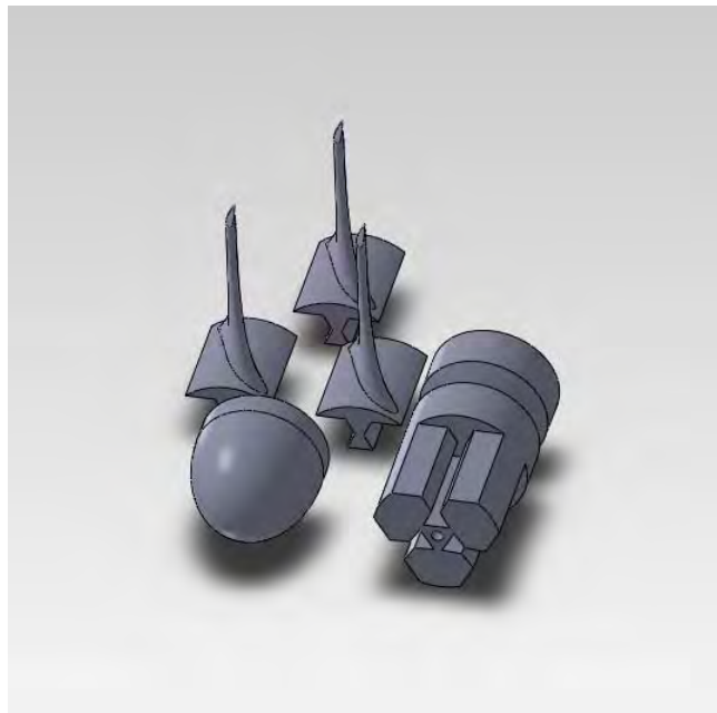
Figure 10: Solidworks model of NACA 4421 foil. Turbine was built as an assemble.
