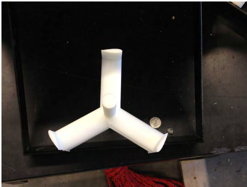
Figure 8: Final Product Vertical-Axis Turbine Top Profile. 5.8 inch diameter, 1 inch chord length, NACA 0020
