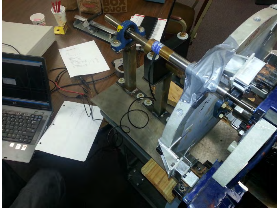
Figure 31: Experimental setup for measuring force at different engagements.
