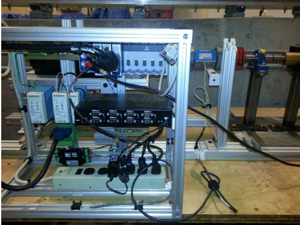
Figure 33: Data acquisition board that allowed for data to be recorded.
