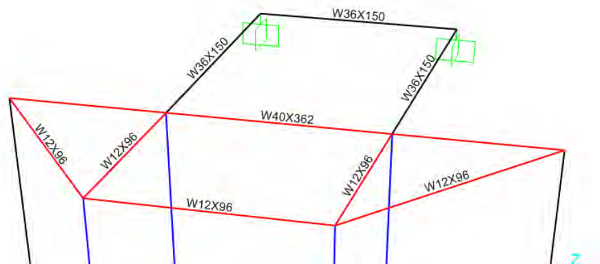
Figure 50: Top-level member sizes.
