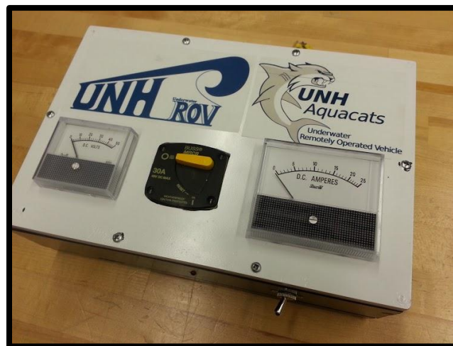
Figure 10: Fuse Box with switch, ammeter, and voltmeter.
