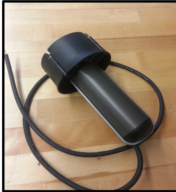
Figure 18: Seabotix BTD 150 DC brushed thrusters.
