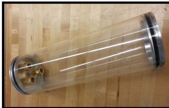
Figure 12: Tube, end-cap, o-ring, and bulkhead fitting assembly.
