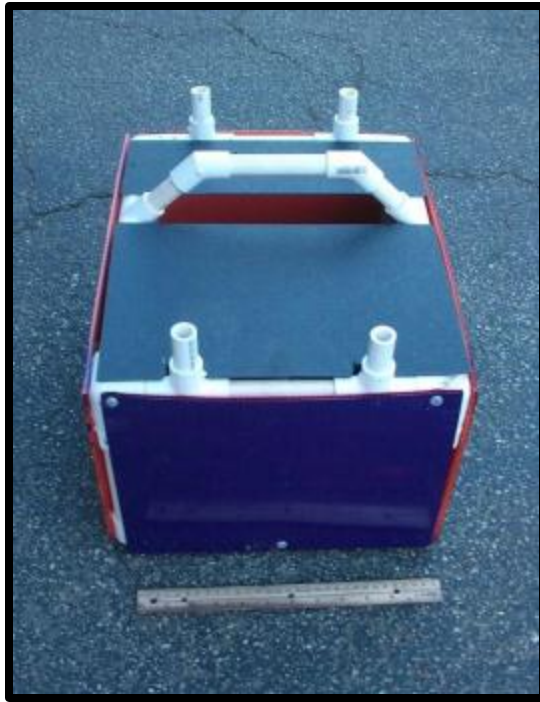
Figure 3: Transmissometer mounting platform without rotating disk.
