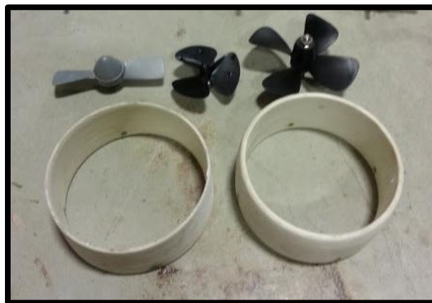
Figure 16: Propellers and cowlings used in thruster testing.
