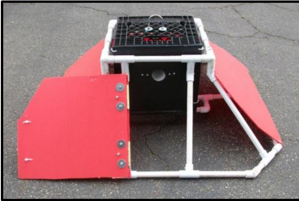
Figure 2: Backbone Interface Assembly PVC construction.
